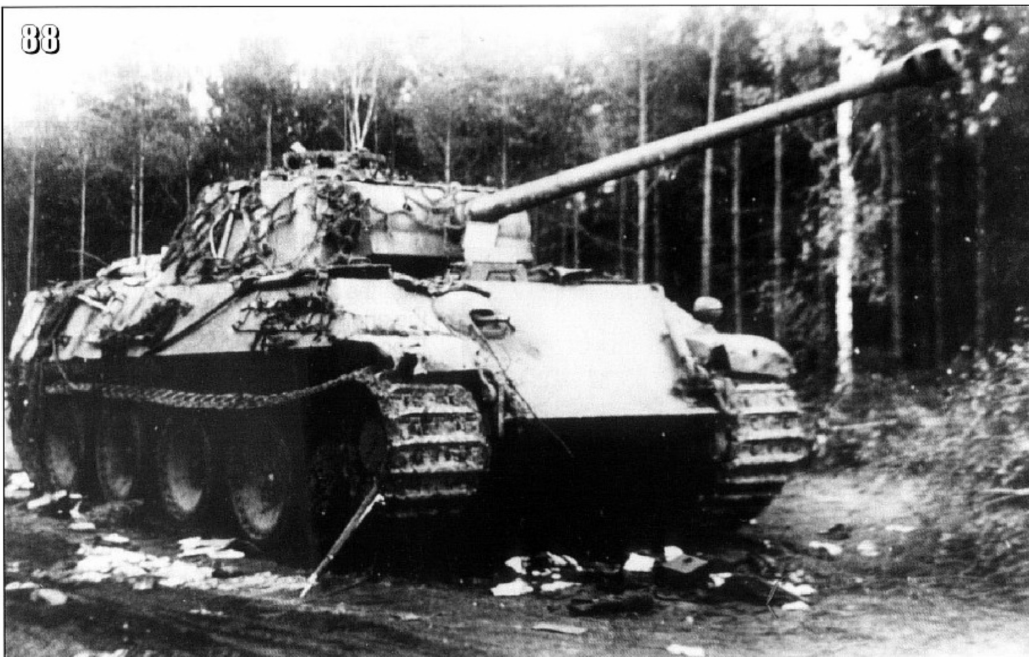
88- A Panther near Berlin in April, 1945. This Ausf. G was brand new. Towards the end of the war many tanks left the factory with incomplete fittings and equipment missing. (Anderson)
