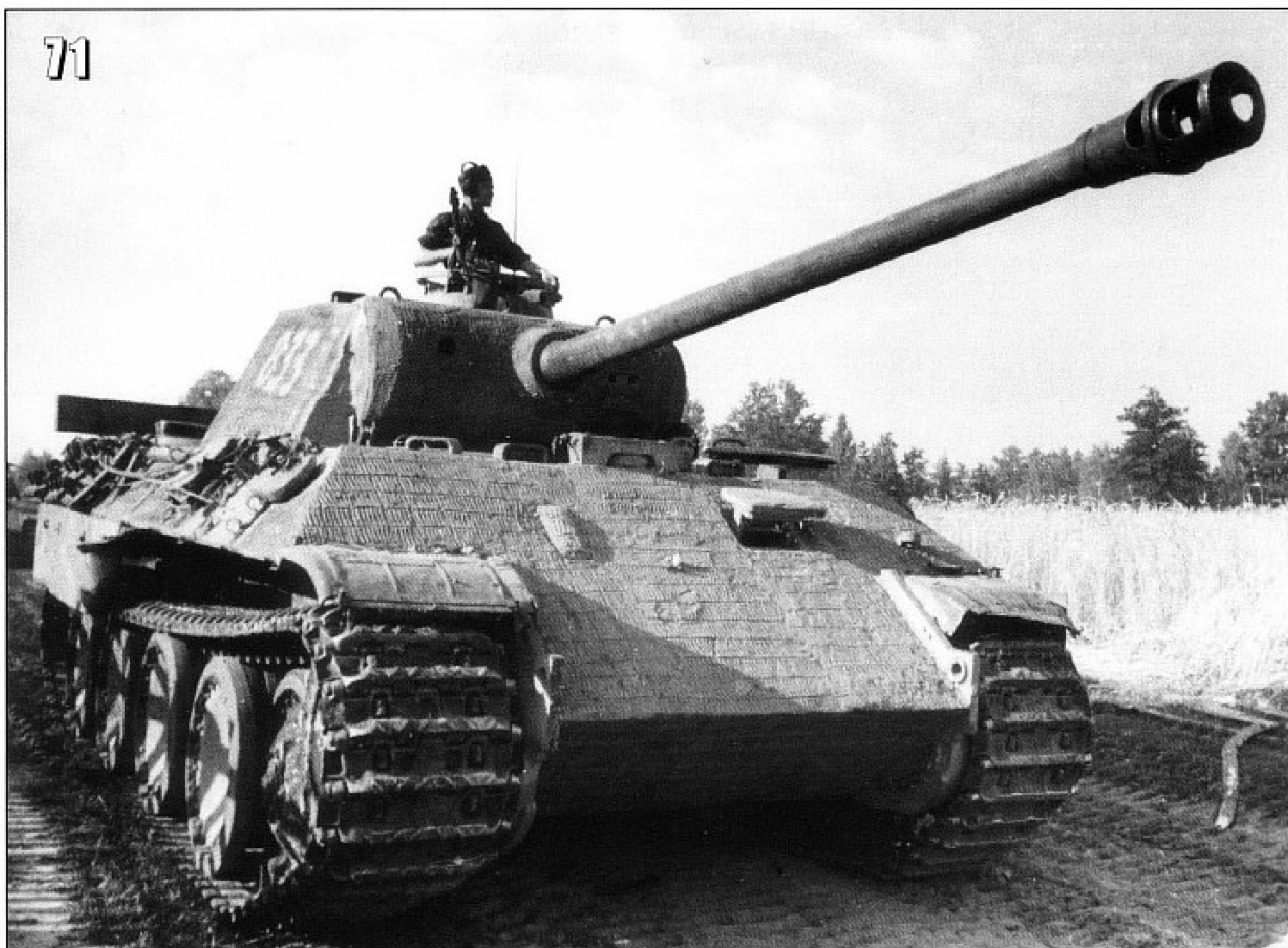
71- Tank "833" was a powerful machine! Note the Zimmerit applied on this early Ausf. A. The left headlight is gone as are the side armours. Only the brackets are still in place. (Anderson)
