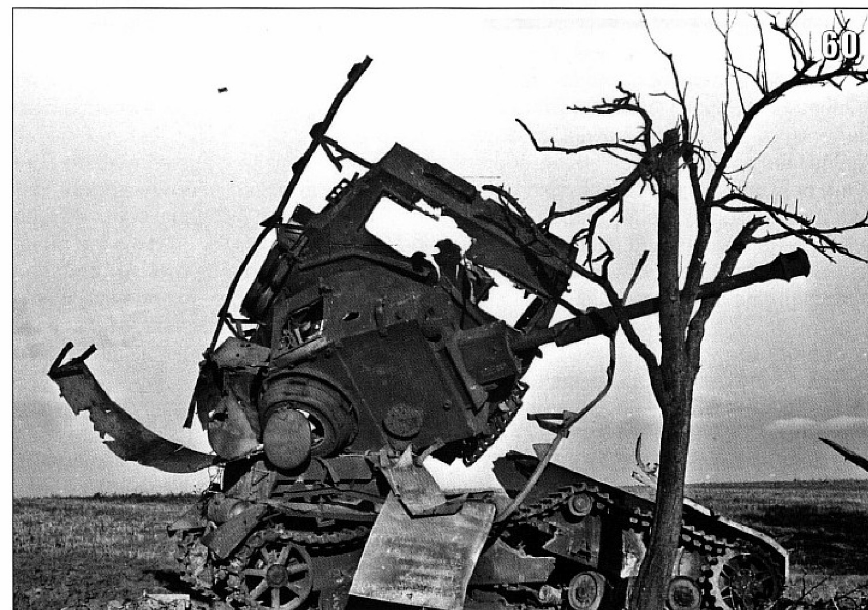
60- This Panzer IV was destroyed by an internal explosion. The upper part of the hull and the turret were blown to bits. (Y. Kadari)
