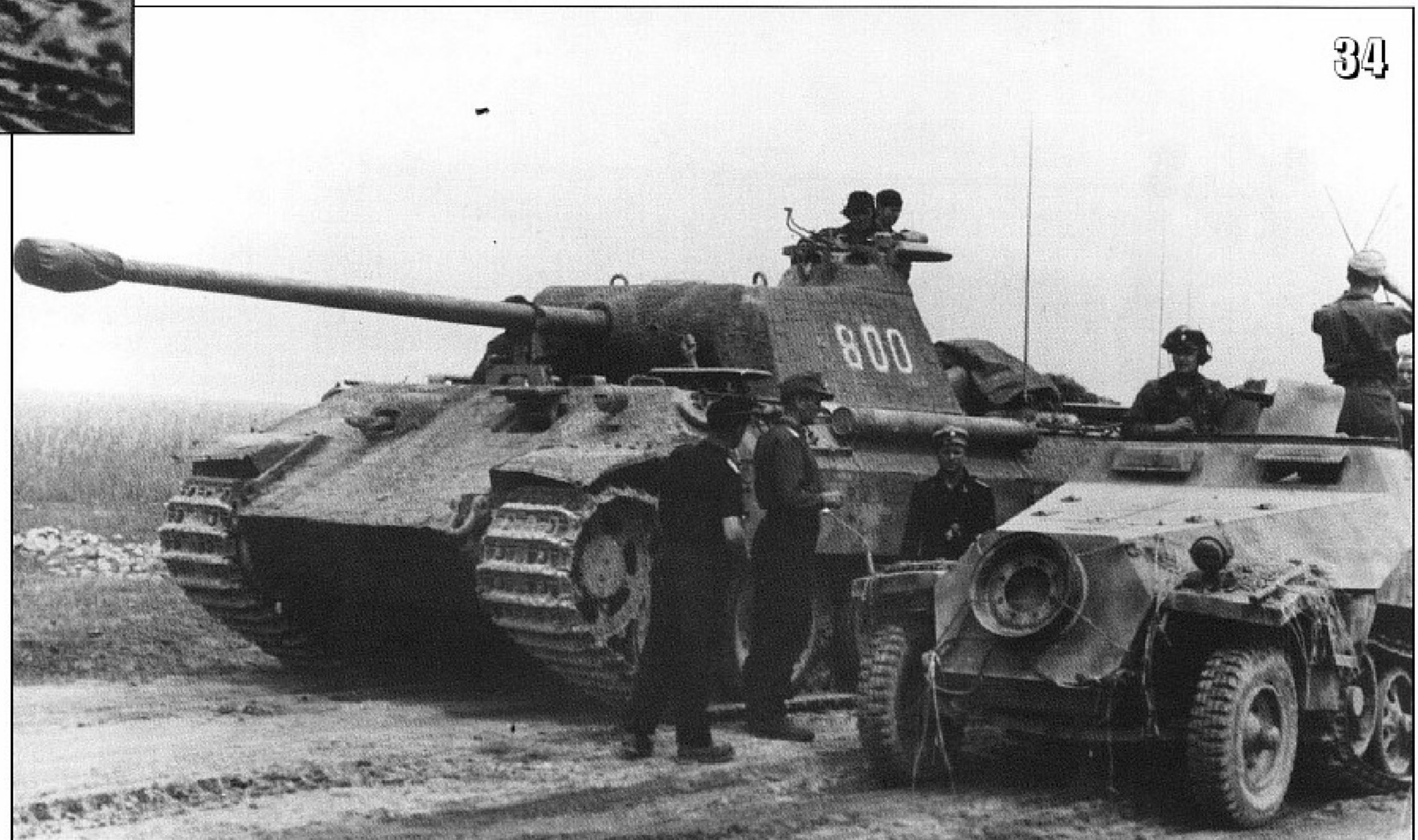
34- The 8th Tank Company Commanding Officer briefs the commander of a Panzergrenadiere Company on the field. By its tactical code (800) this Panther Ausf. A is a command tank. Unusually, it does not have any extra aerial installed. Both the vehicles in this photo have suffered some light combat damage. (R. Michulec)
