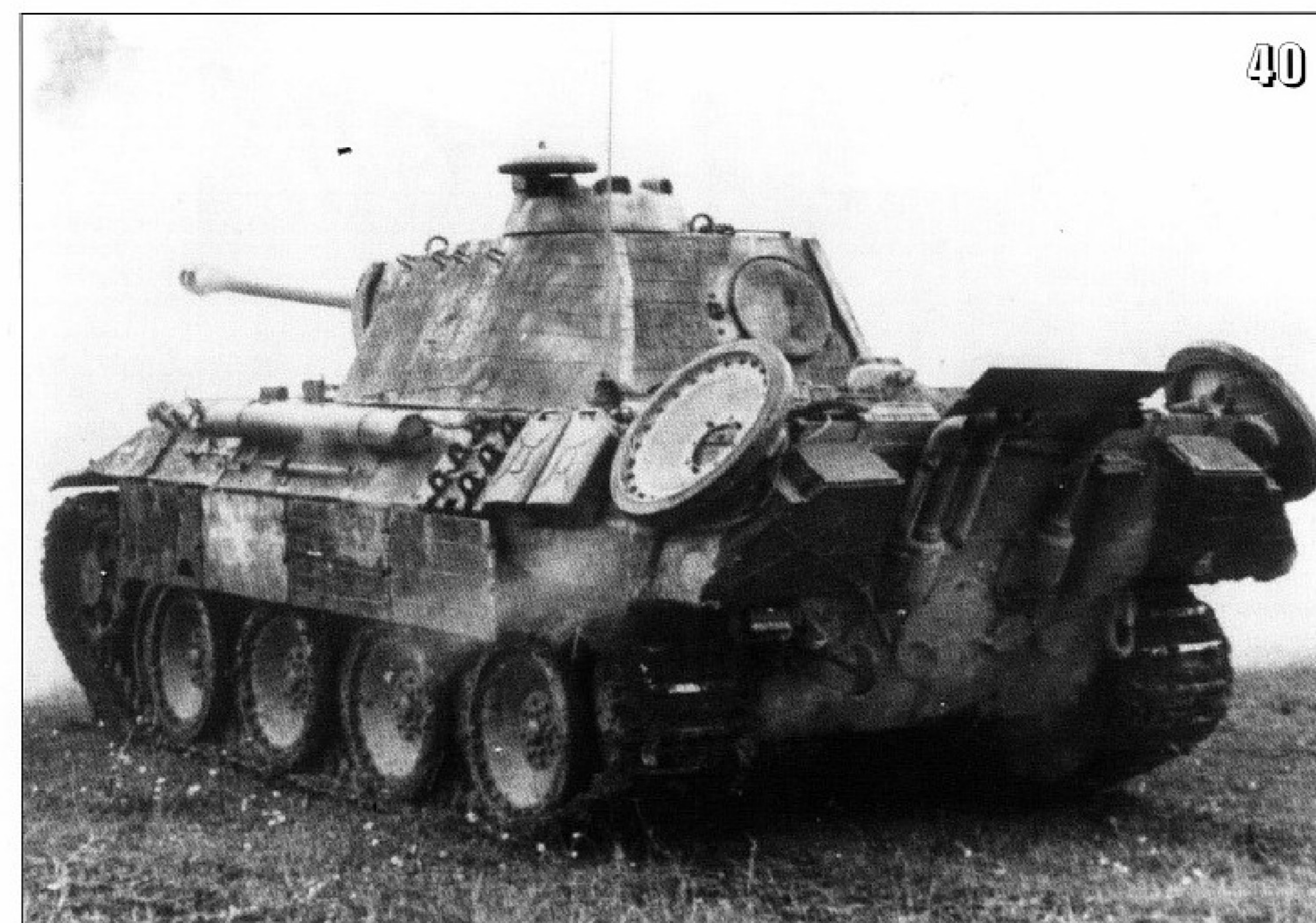
40- This Panther, belonging to Pz.Gren.Div "Grossdeutschland" was photographed near Wilkowschken, during the Autumn of 1944. Note the camouflage pattern and Zimmerit compound applied on this late Ausf. A. The turret is fitted for the spare track sections. Two spare running gear wheels are carried on the rear sides of the hull. (Anderson)
