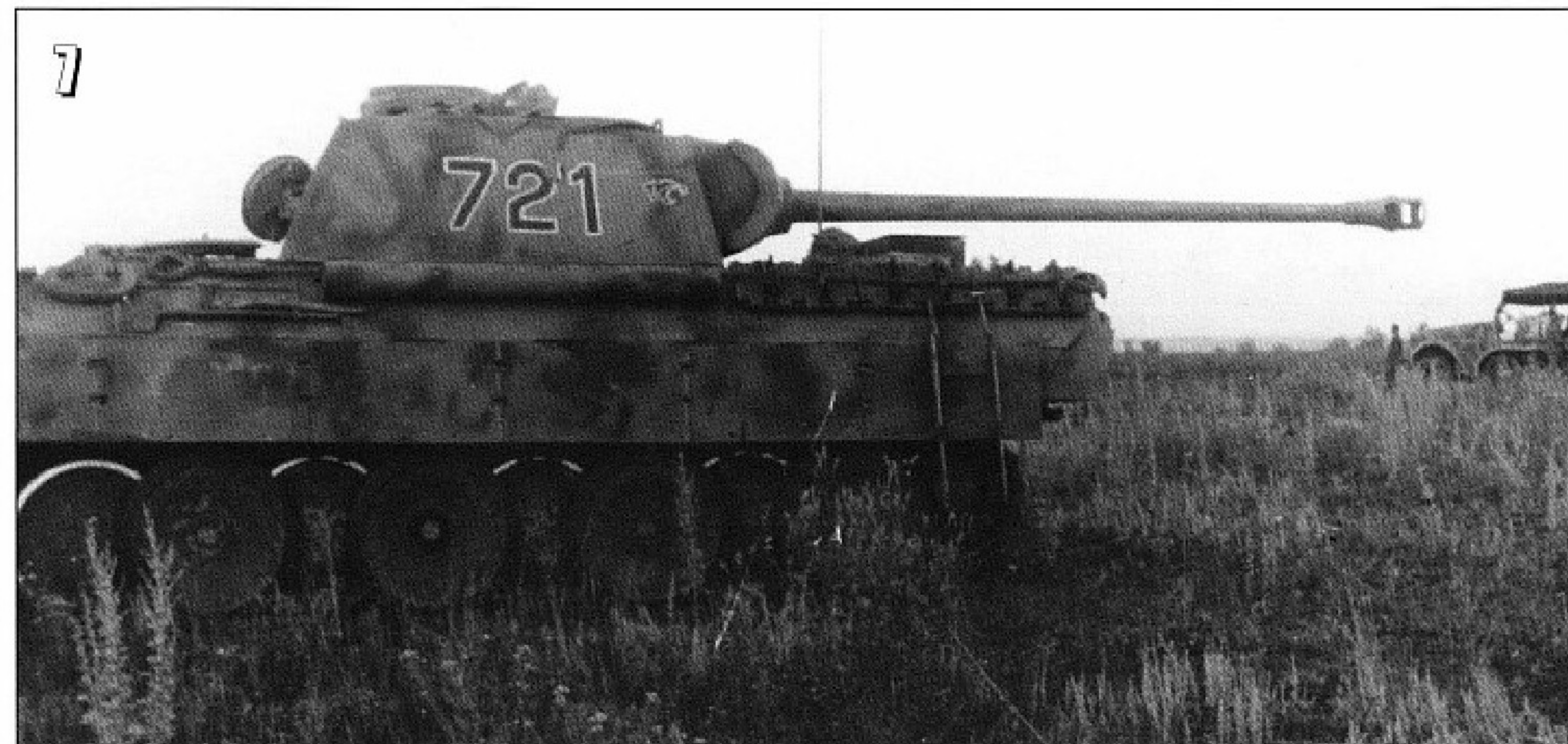
7- Pz.Abt. 52's tank number 721 at Kursk, showing many of the characteristics of the early production. The Zimmerit compound has not been applied and the turret bears the outfit distinctive insignia, a wide open mouth panther. The camouflage is a pattern of irregular dark green stripes on a dark yellow base. Note how the tracks have polished the edge of the rim of the roadwheels. (J. Wilhelm)
