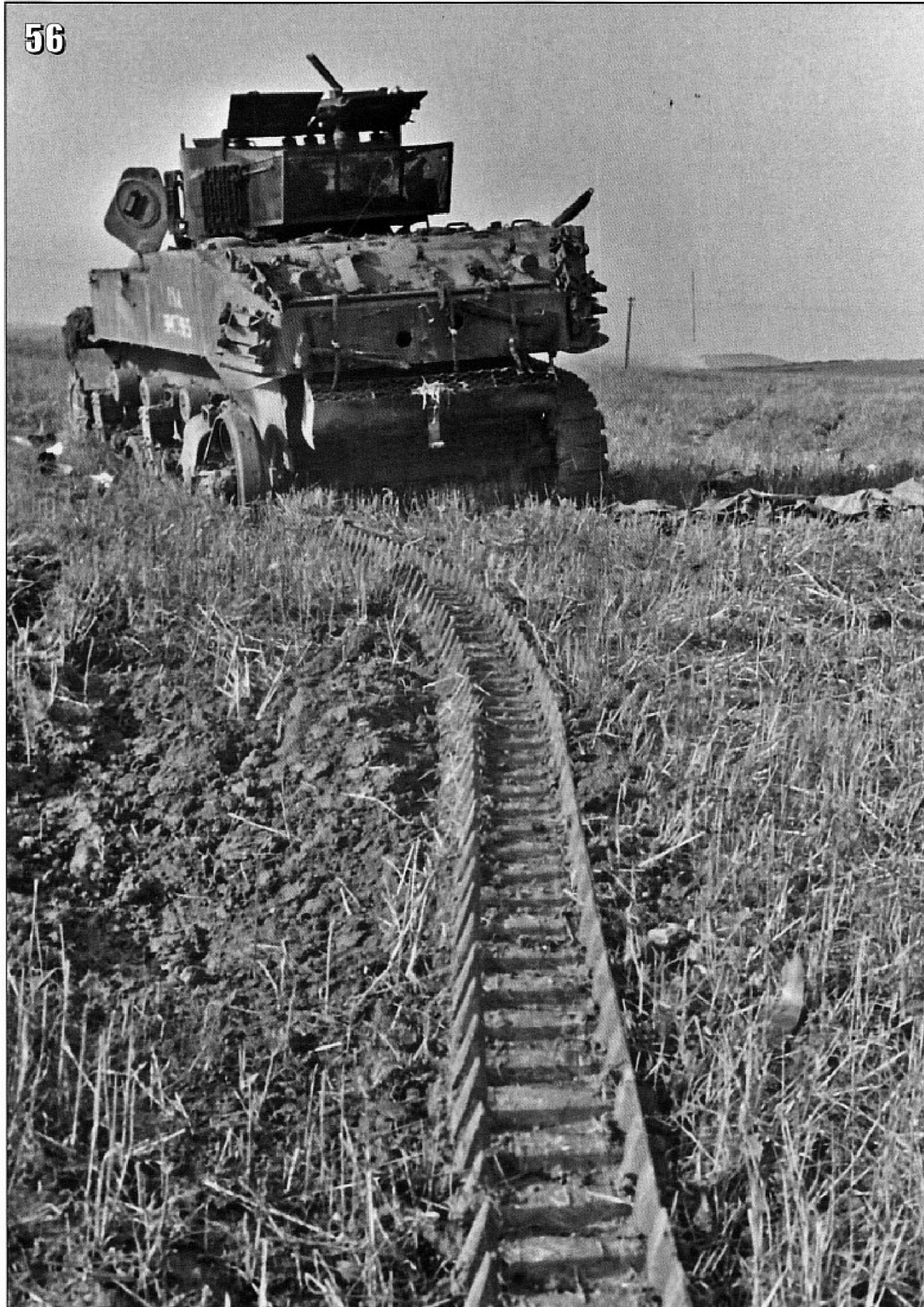
56- This M5 was hit twice in the rear part of the hull. Note the field made turret basket. (Y. Kadari)
