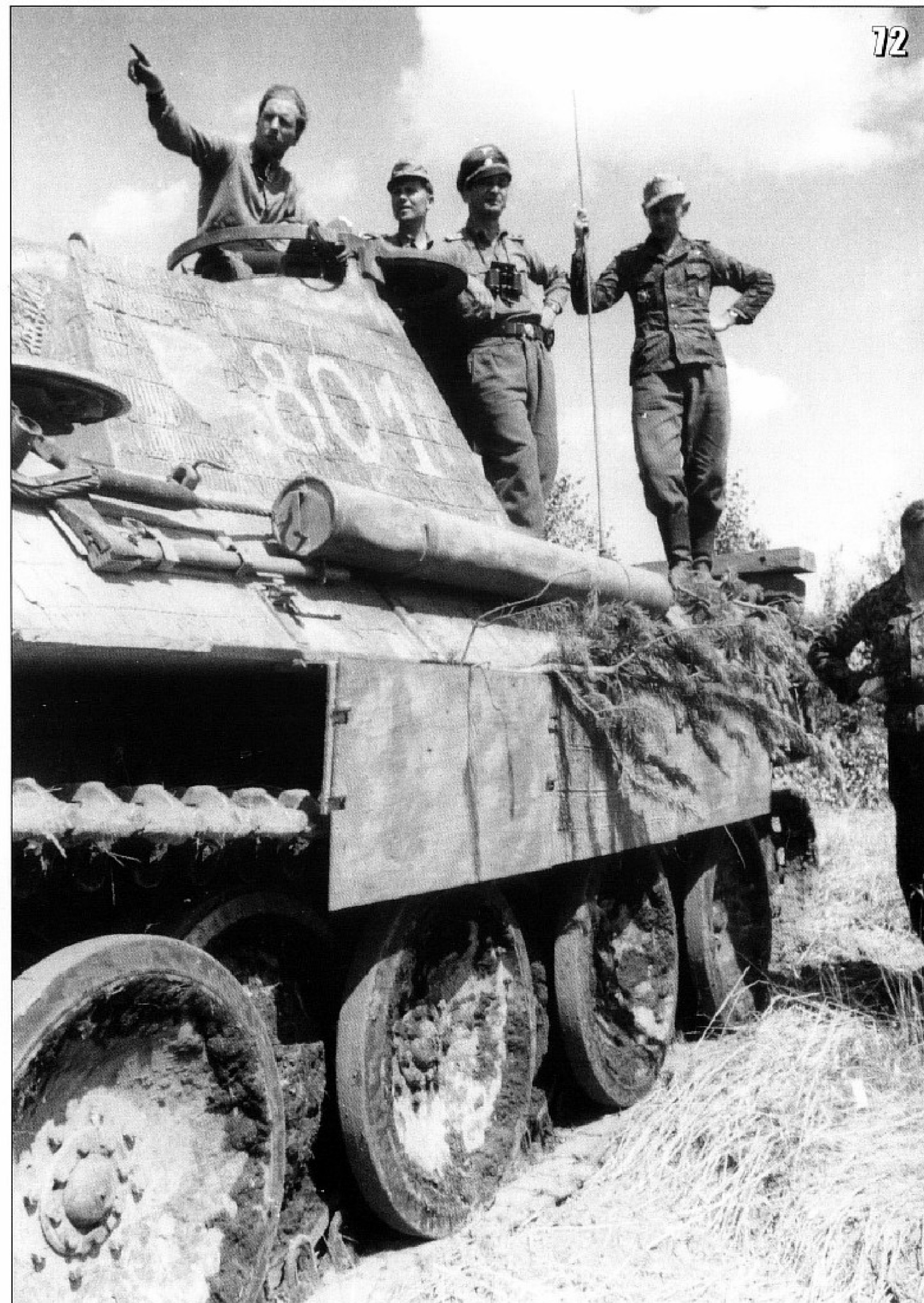
72- Officers briefing. This Ausf. A has mud plastered roadwheels and only part of its side armours left. The turret Zimmerit coat is chipped in several places and the usual pieces of timber are carried on the engine deck. (Anderson)
