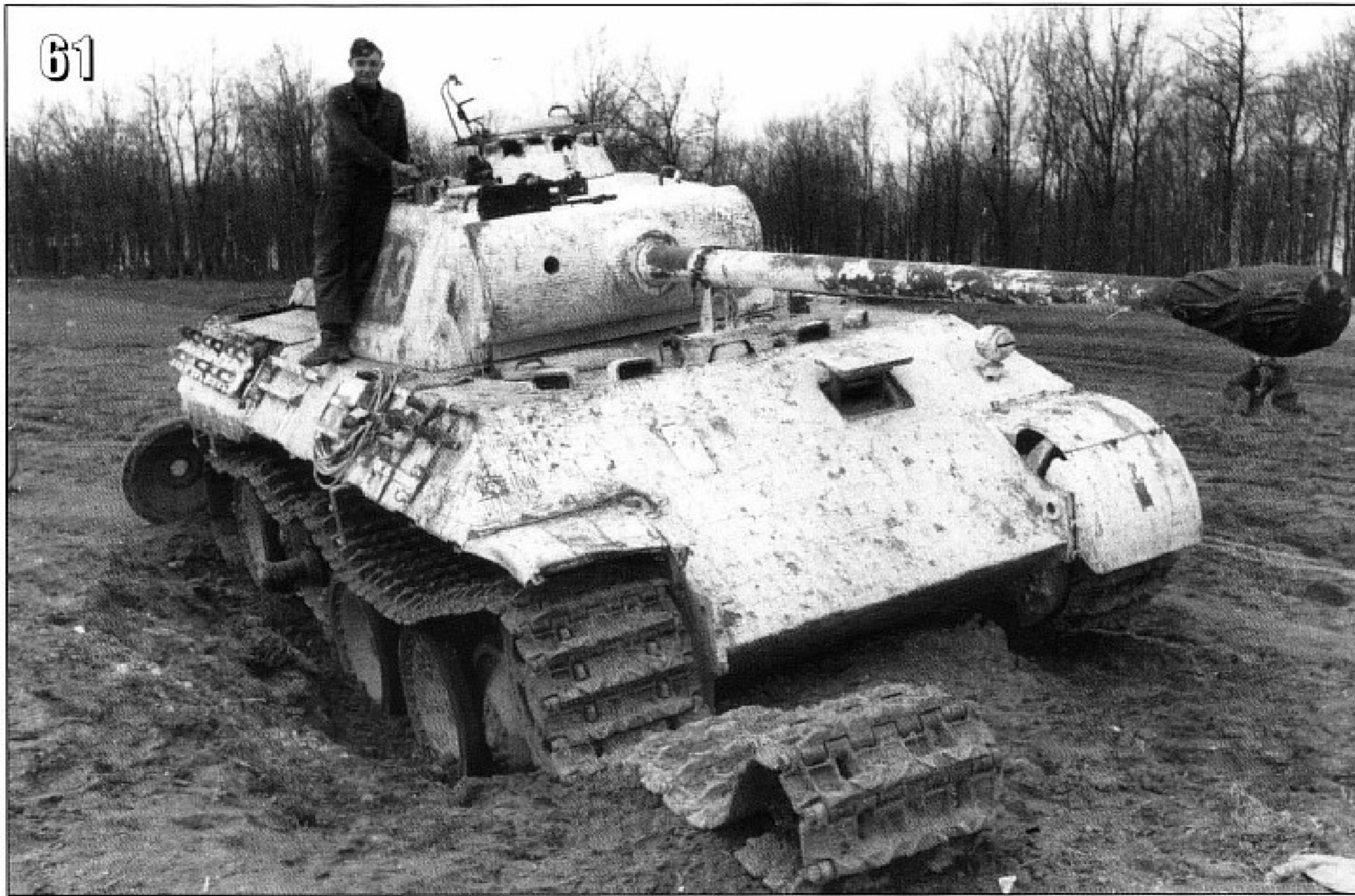
61- A Panther Ausf. A belonging to the "Wiking" Division on the Eastern Front. Looks like an AT mine has caused extensive damage to the right running gear which will require a long time off the line to repair. Use of landmines was particularly effective against German AFVs. (Anderson)
