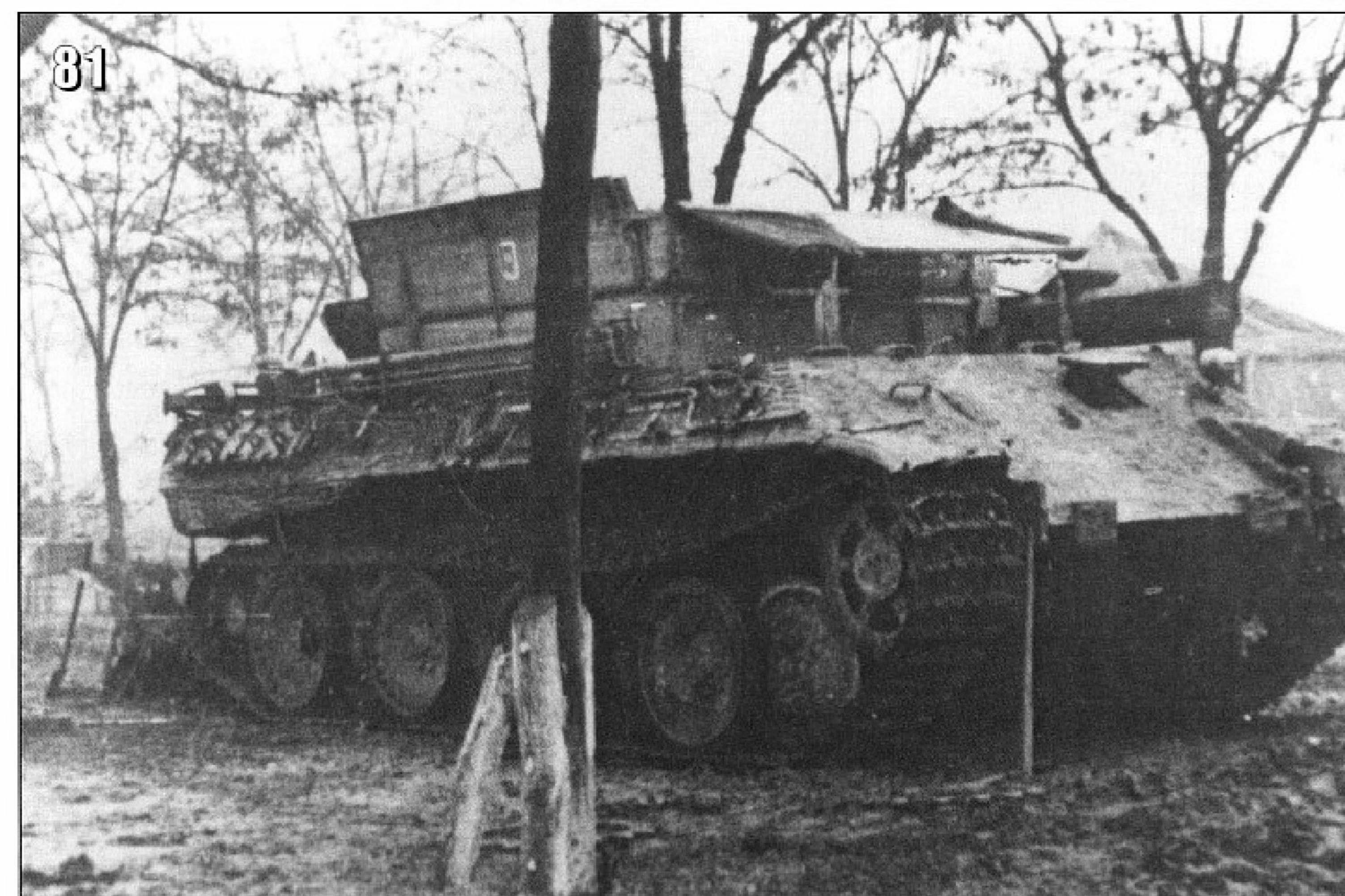
81- The Bergepanther was a very efficient recovery vehicle. Production of standard AFV was prioritised over that of this specialized version of the Panther. Besides its towing capacity, the Bergepanther was fitted with a boom crane and a hull mounted 40 ton winch that could be increased to 80 ton. (M. Kolomietz)
