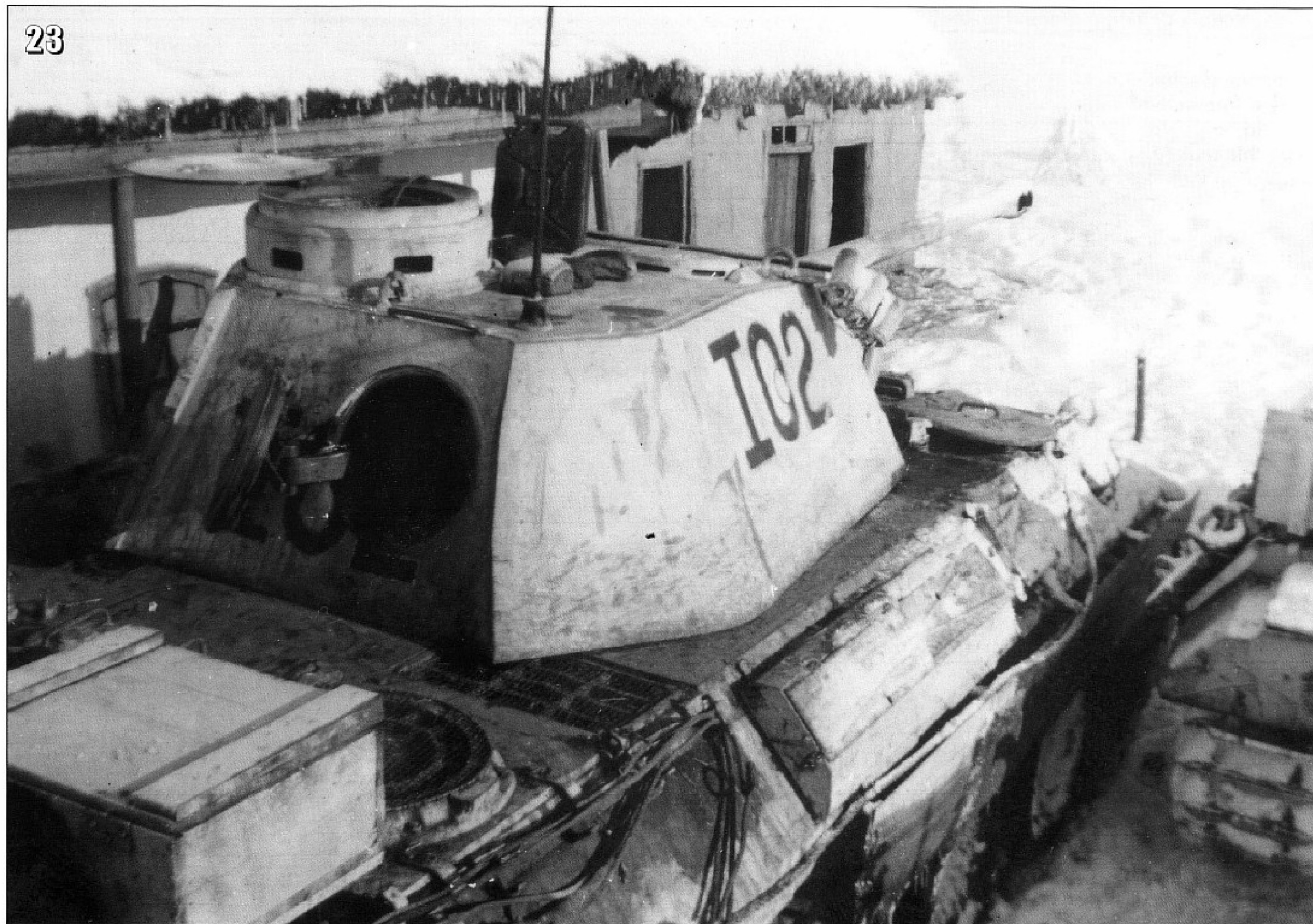
23- Tank "I 02", a Pz.BfIs.Wg Panther, displays all the characteristics of the early Ausf. D's. The smoke dischargers and the side toolbox are present. The additional wireless aerial is installed on the turret roof. Some large wooden crates are stowed on the engine deck. (J. Wilhelm)
