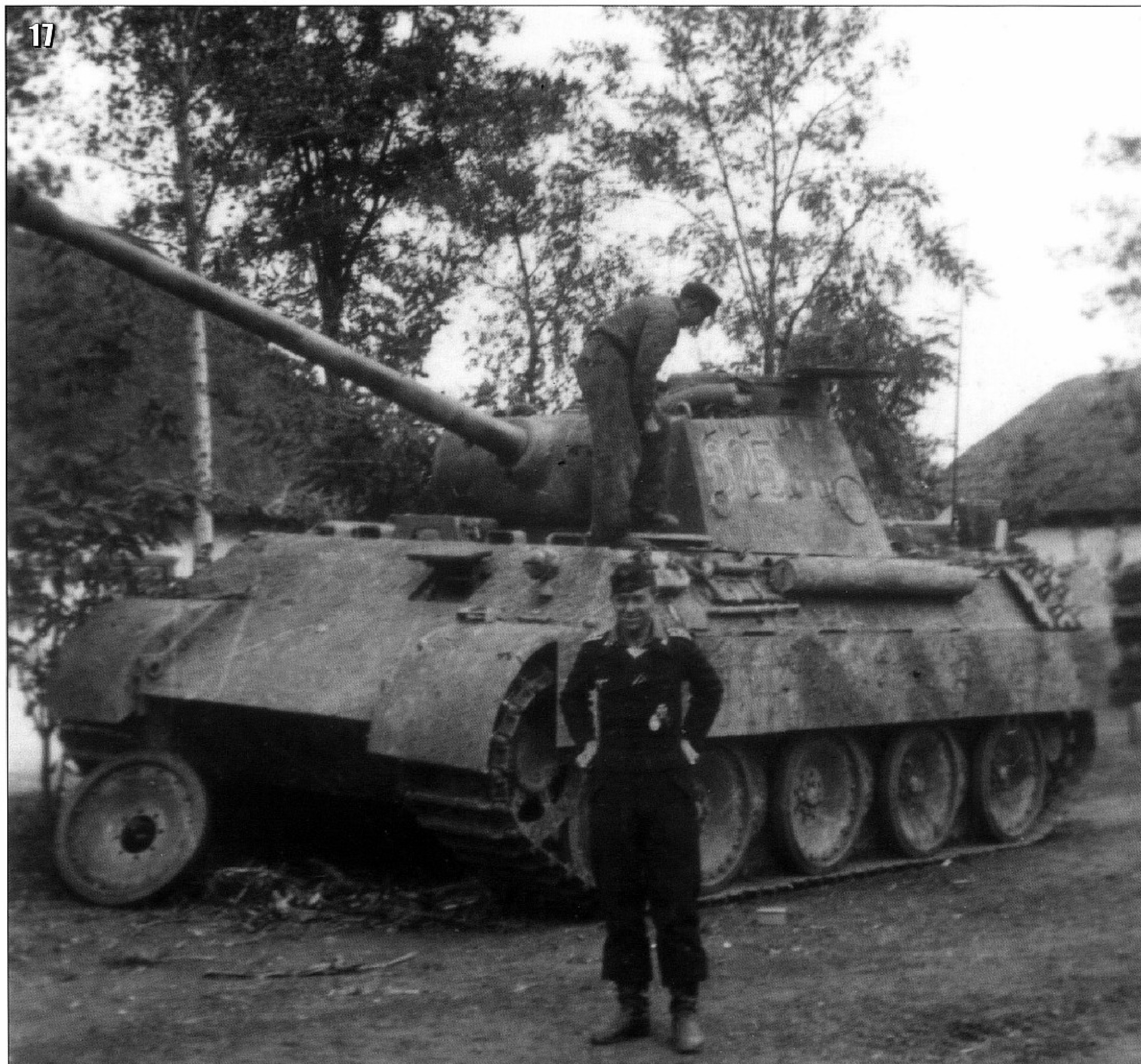
17- A nice photo of a late Ausf. D, built after July, 1943. The side aprons are covered with Zimmerit compound. Unusually, tactical codes on the turret are painted over. A number of brackets have been welded on the turret side to support track sections, a common expedient to improve the thin side armour. (D. Terlisten)
