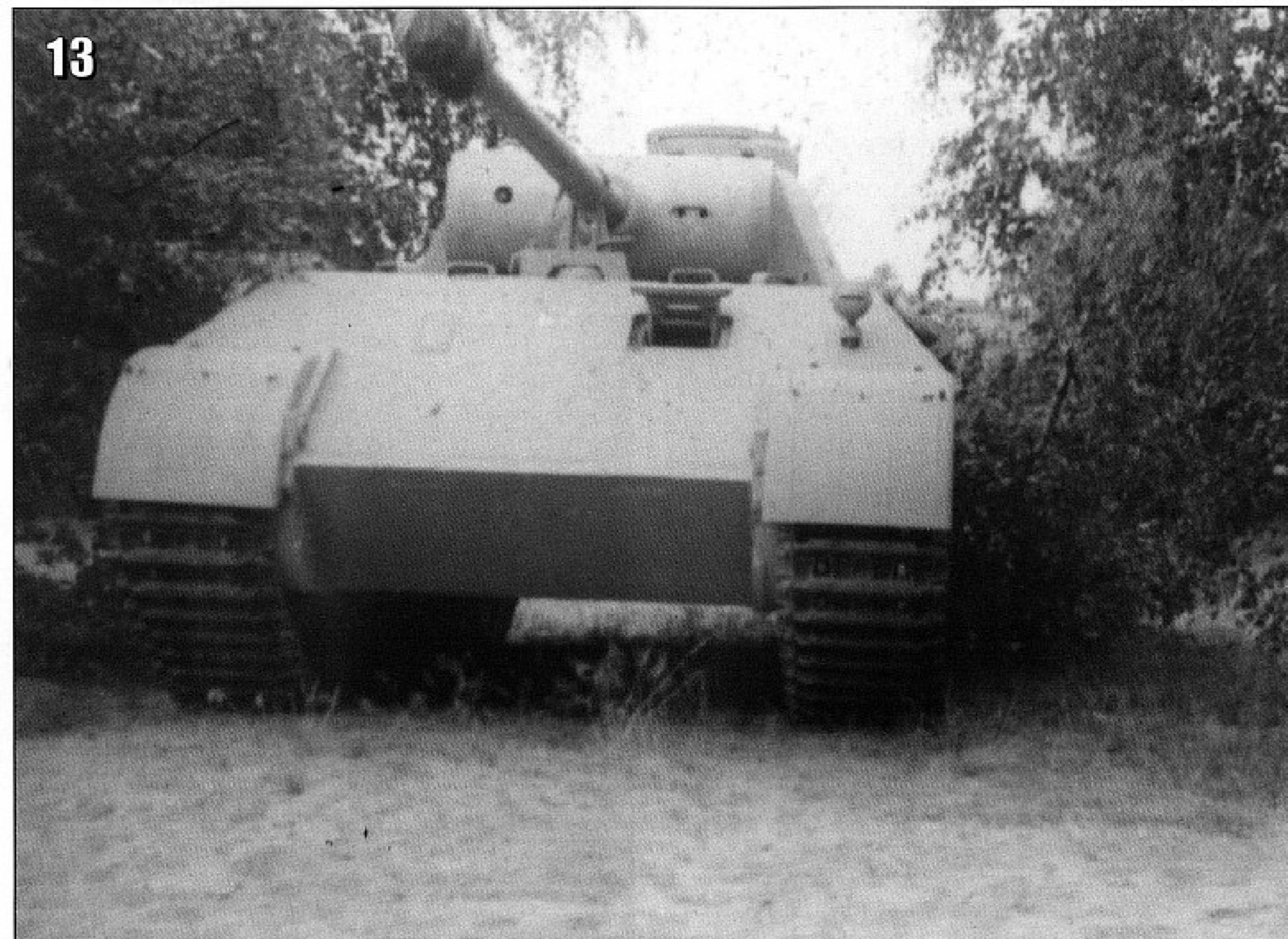
13- A late Ausf. D Panther in the summer 1943. The right headlight and the smoke dischargers brackets are missing. A rail for the AA MG34 is installed on the tank commander's cupola. This tank, which does not sport a camouflage paint job, is probably just being delivered. (S. Clark)
