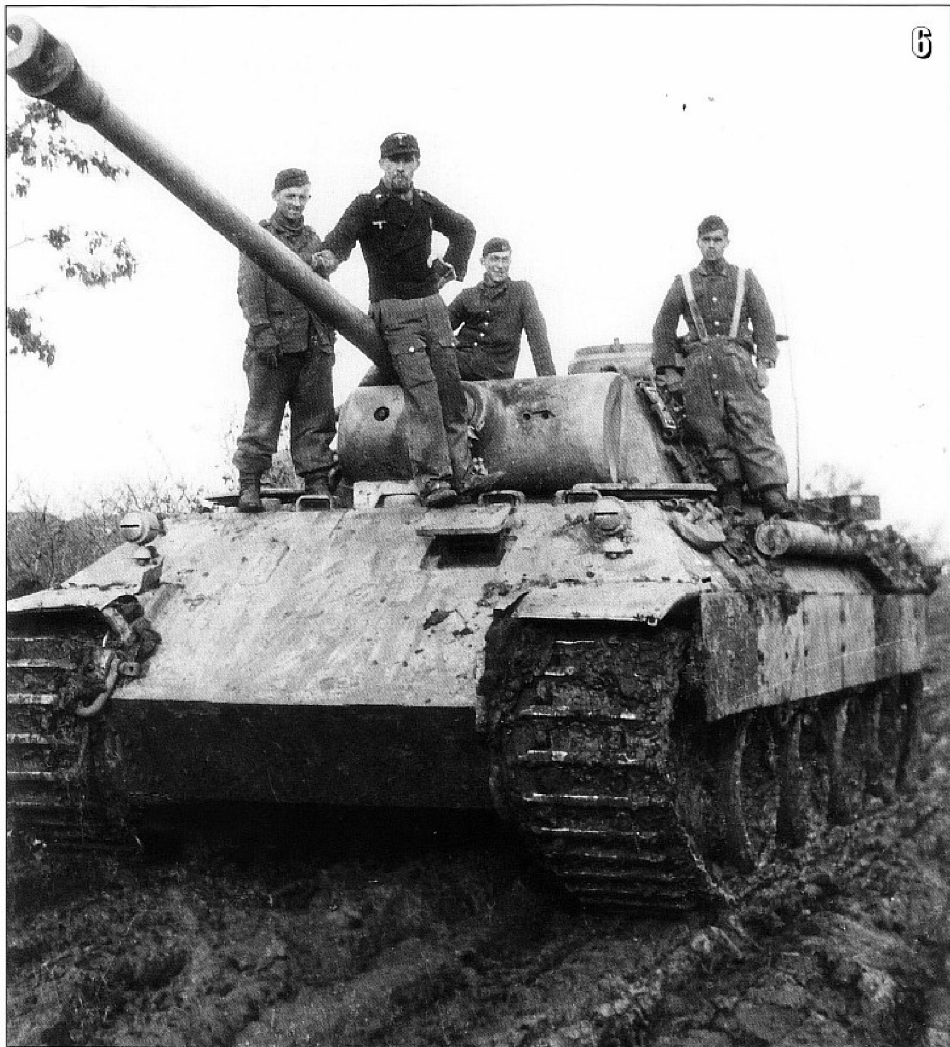
6- Out to the field! The crew of this Panther from either, Panzerabteilung 51 or 52, looks like it is waiting for some action. On the mantlet there are the two holes for the binocular aiming scope. The first 250 Panthers left the factory with the Maybach HL210 engine, which turned out not to be powerful enough for this large tank. (D. Terlisten)
