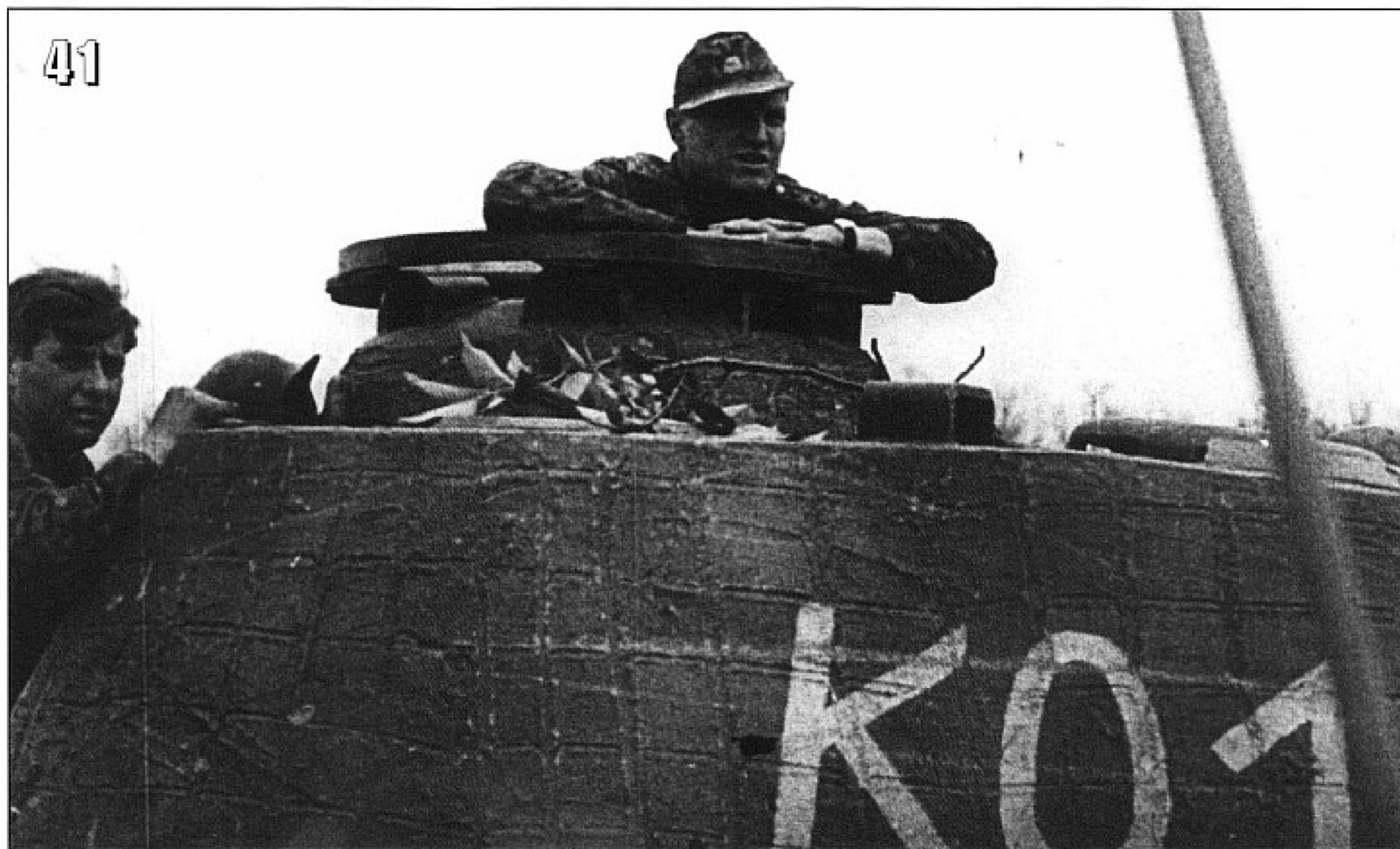
41- Close up of a Panther turret, probably an Ausf. A. This vehicle, coded "K 01" is a command tank as evidenced by the antenna mast. (R. Michulec)
