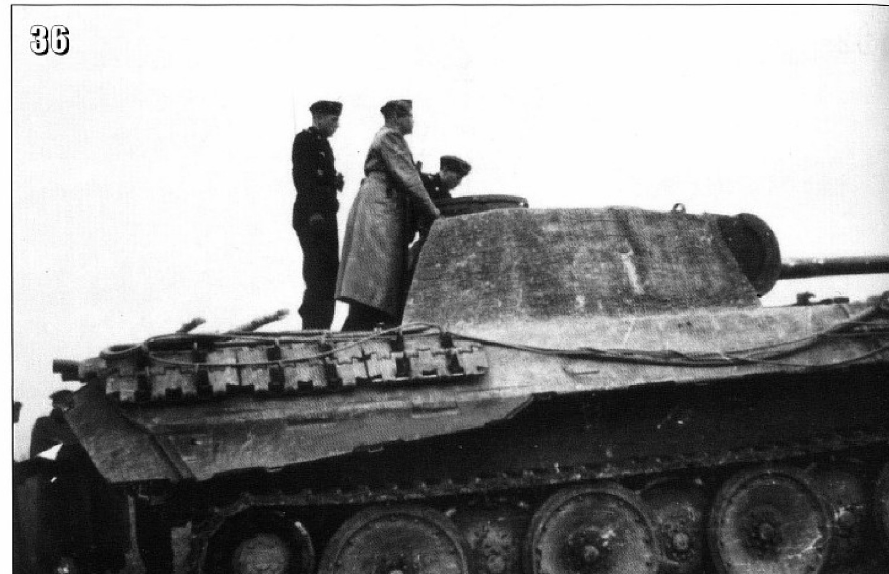
35- A souvenir while on duty for the Fatherland! Four German tankers and their Panther Ausf. A. Even if the tank turret is covered with a tarp, the camouflage pattern is clearly visible. The side armours are missing but their brackets are plainly still in place. (D. Terlisten)
