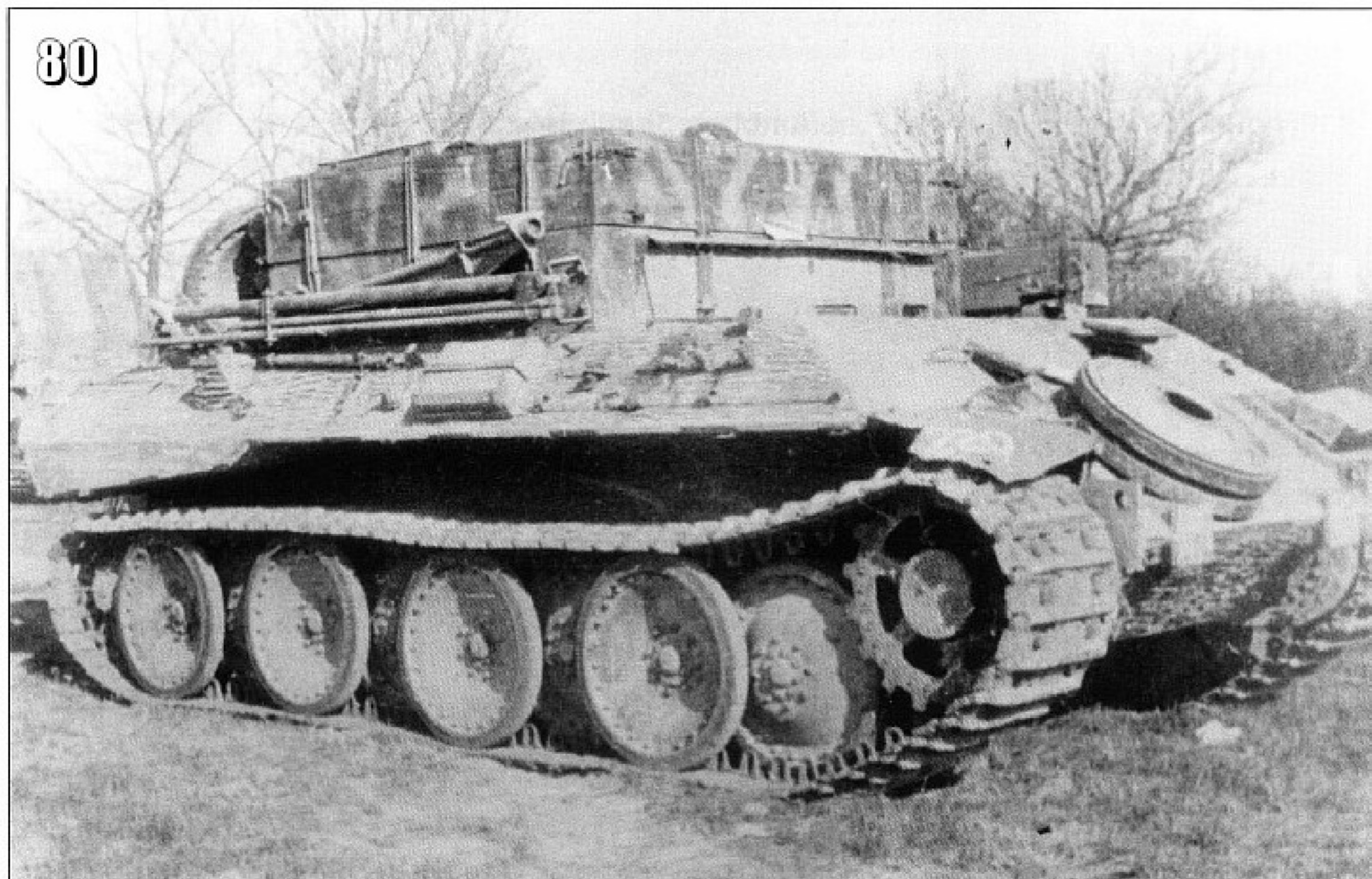
80- The Bergepanther recovery tank, was the most important member of the Panther family. This was the only example of purpose built, recovery vehicles in Germany during WWII. A Bergepanther was powerful enough to tow a Panther or Tiger I or II. (M. Kolomietz)
