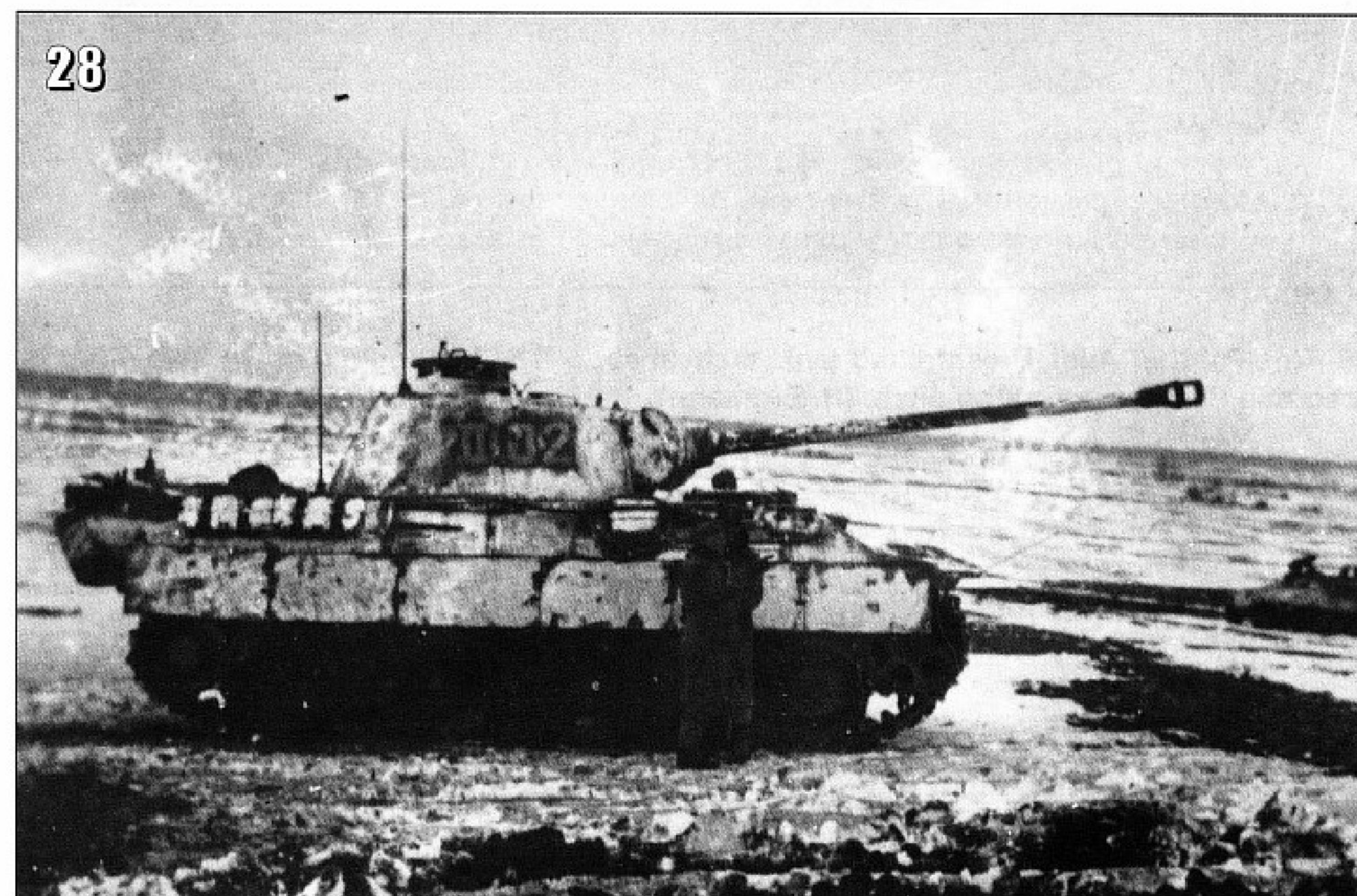
27- Another Ausf. A during the winter of 1944. The mud plastered running gear would indicate that snow is melting, transforming Russia into a mud hole hampering military operations for a long time. If the temperature dropped, the Panther running gear could be blocked by frozen mud. The front fenders look unusually larger on this tank. (J. Wilhelm)
