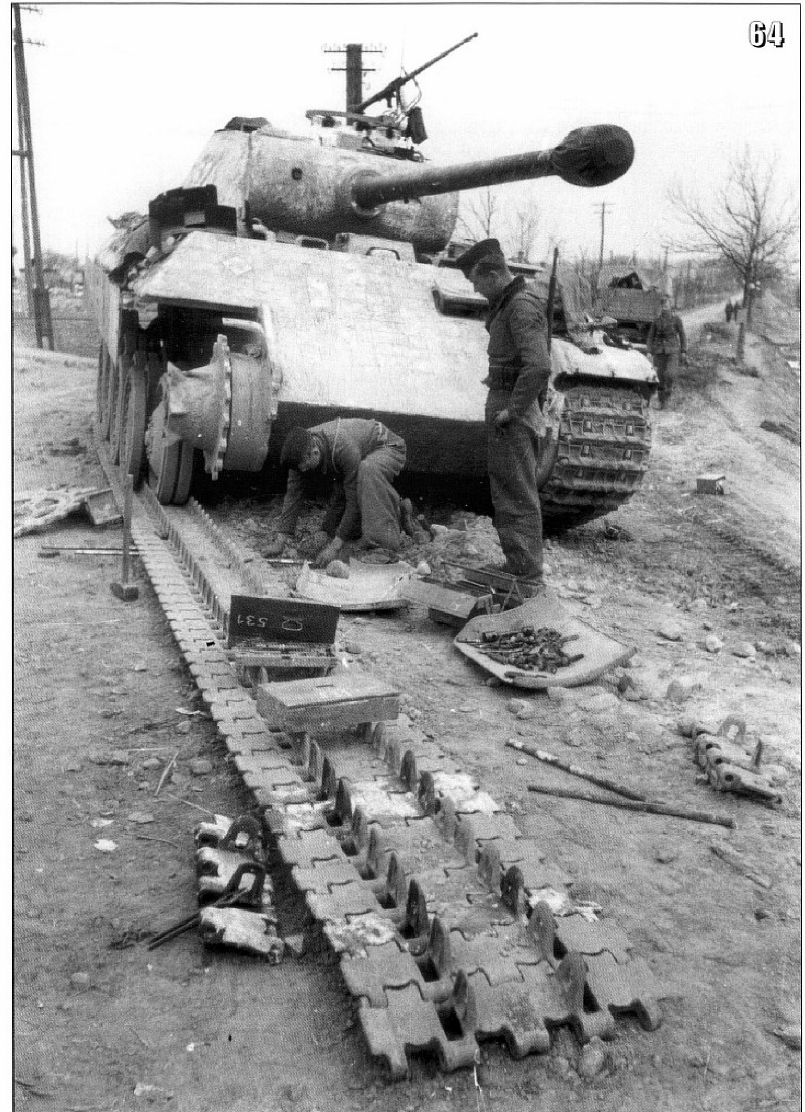
64- Broken tracks..! The crew of this Panther Ausf. A working to repair the sprocket wheel. The weight of the track itself could make this task very difficult to perform. (Anderson)
