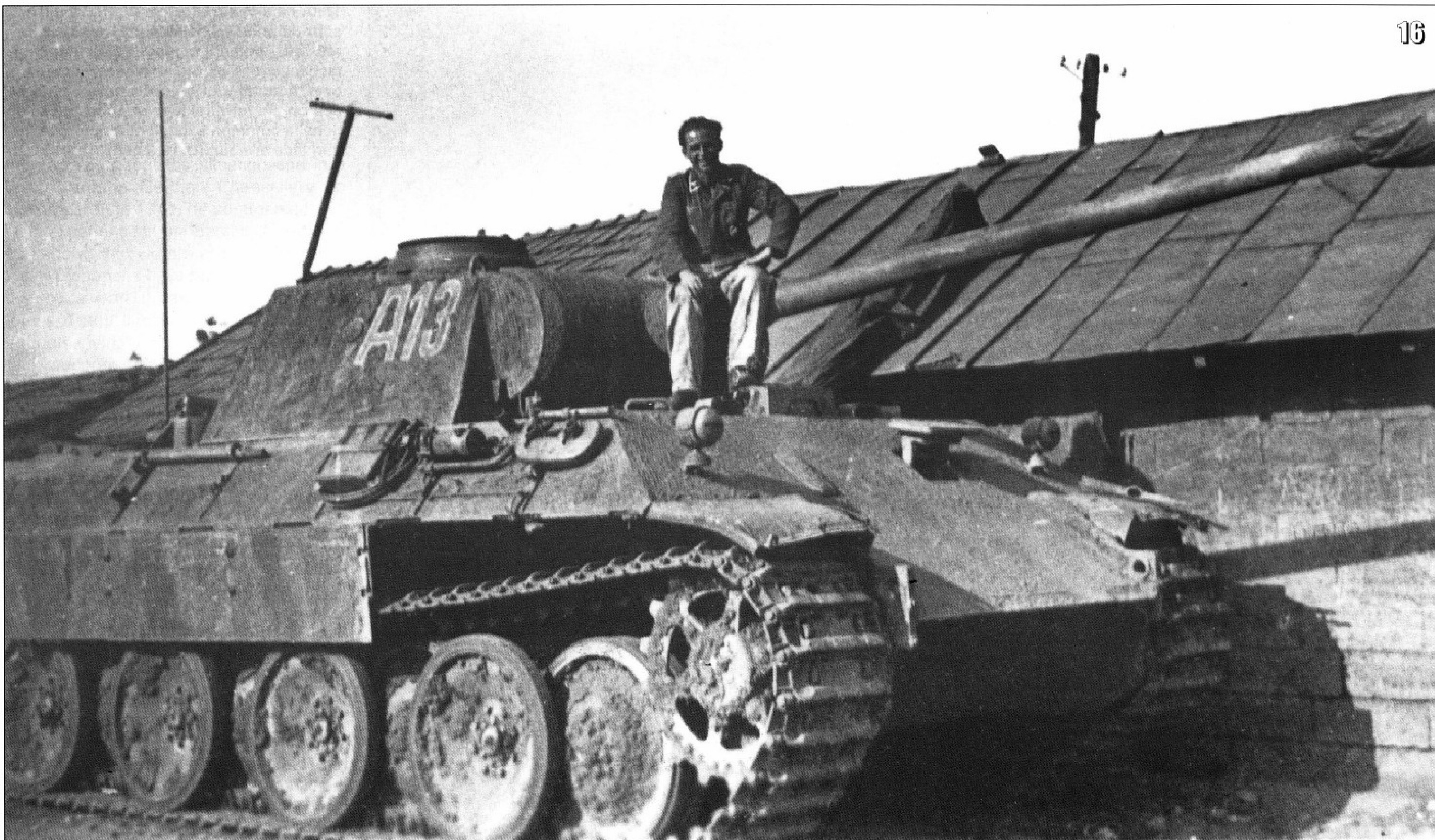
16- Panther "A13" is an early production Ausf. D (no gutters, two headlights, early running gear wheels, no smoke dischargers). This tank has a field applied coat of Zimmerit as it was commonly done after September 1943. The armoured vent is visible on the engine deck. (R. Michulec)
