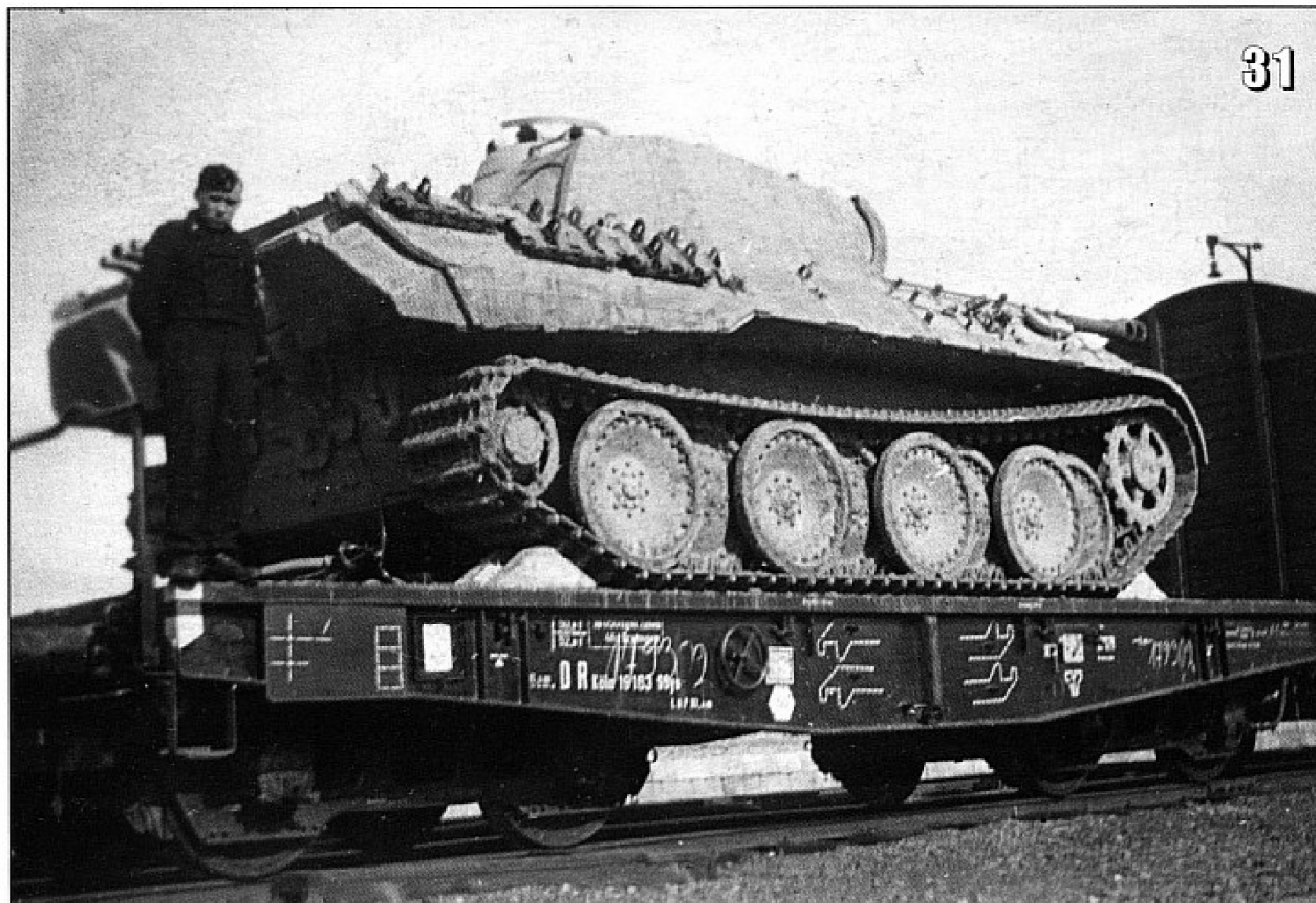
31- A brand new Ausf. A ready to be shipped to the Eastern Front, Spring of 1944. The side armour and their brackets will be installed upon arrival. Panther tanks were exactly as wide as the maximum clearance allowed for railroad transportation. (Verhaaf)
