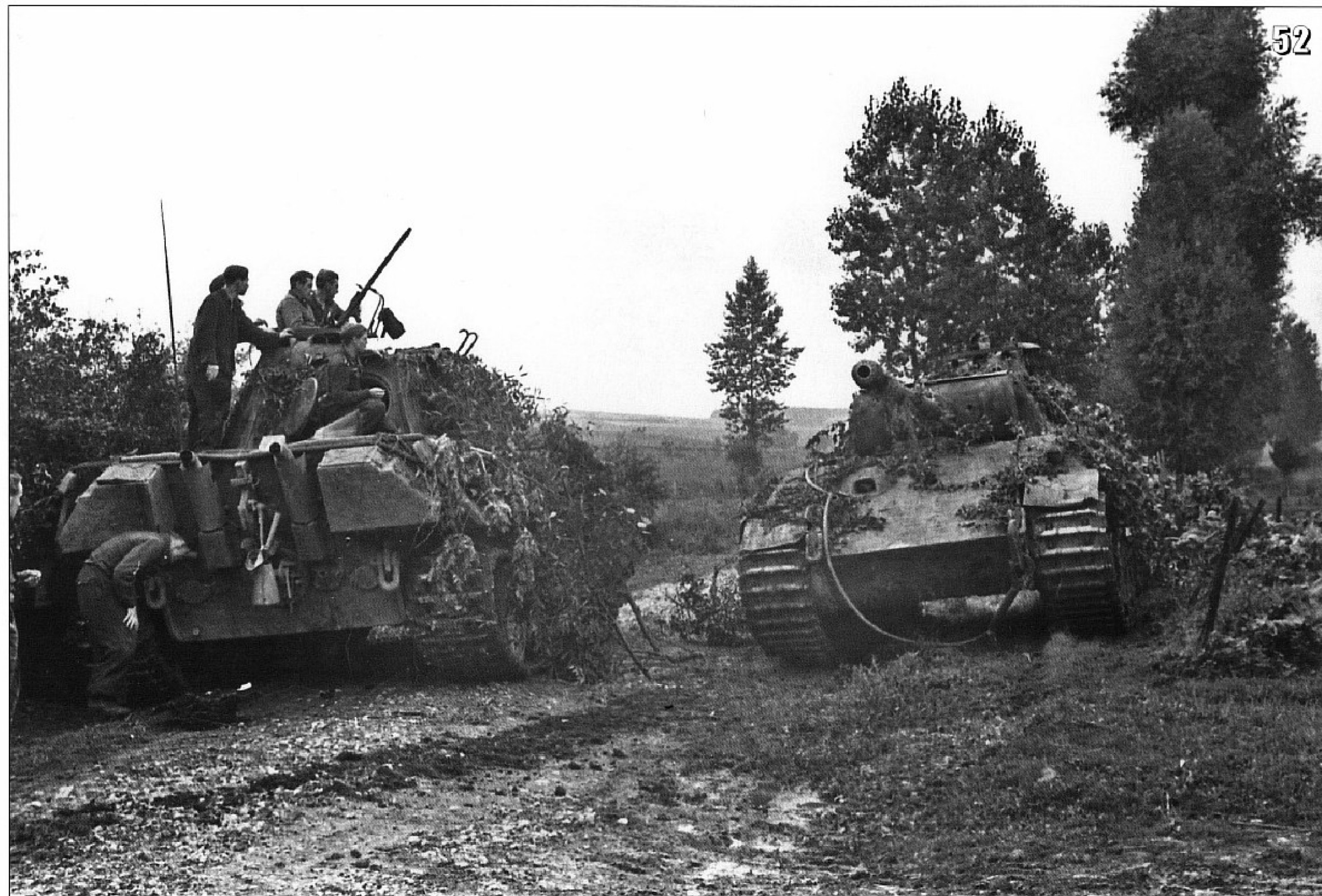
52- Two well camouflaged tanks move carefully from a tree patch to another. The Panther on the left has the AA MG installed, the one on the right has a steel cable fitted to the front towing clevis. (Y. Kadari)
