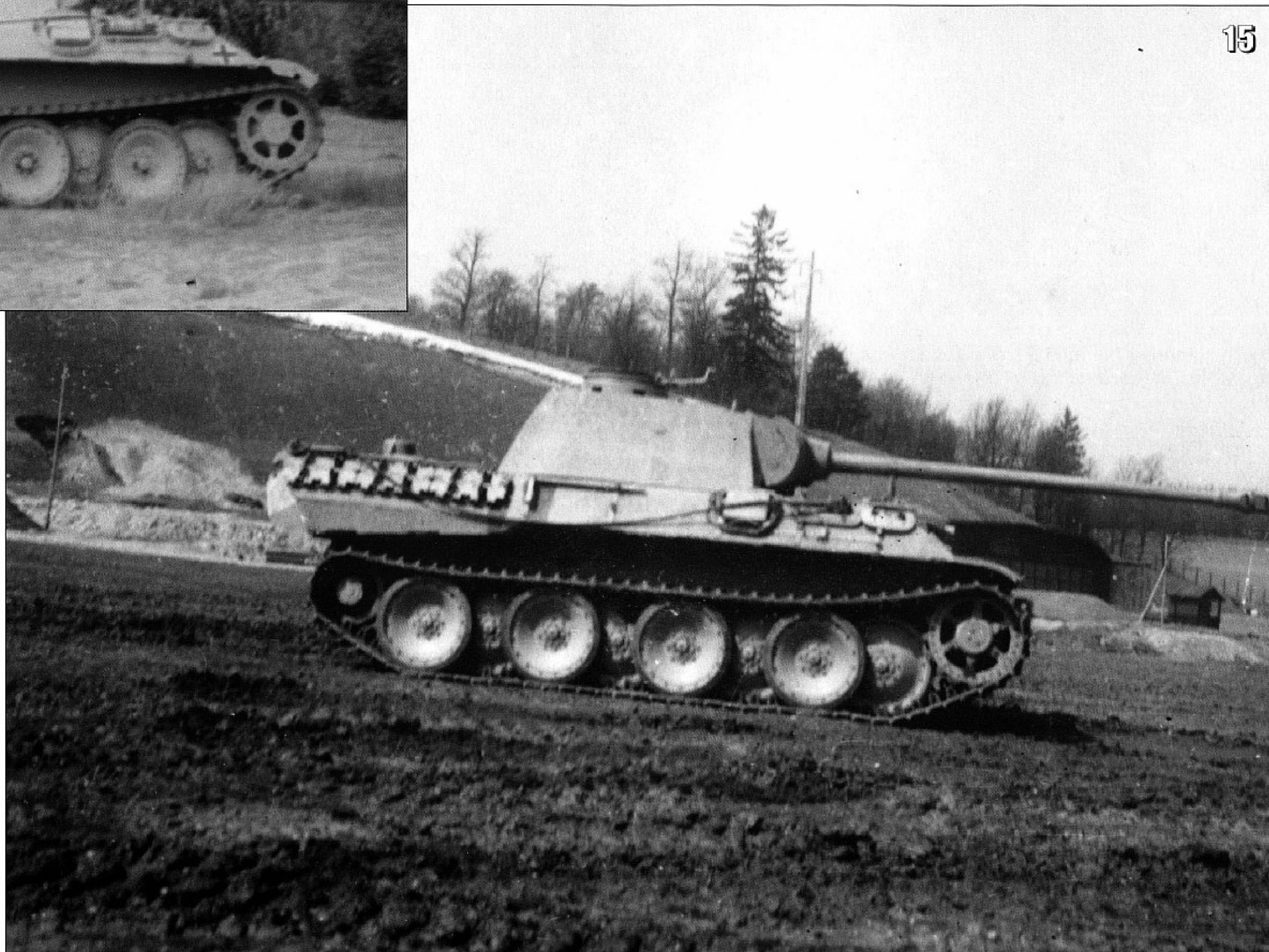
15- The lack of the side armoured aprons and the armoured vent outline on the rear deck are in evidence on this, run of the mill, mid production Ausf D. (M. Zöllner)
