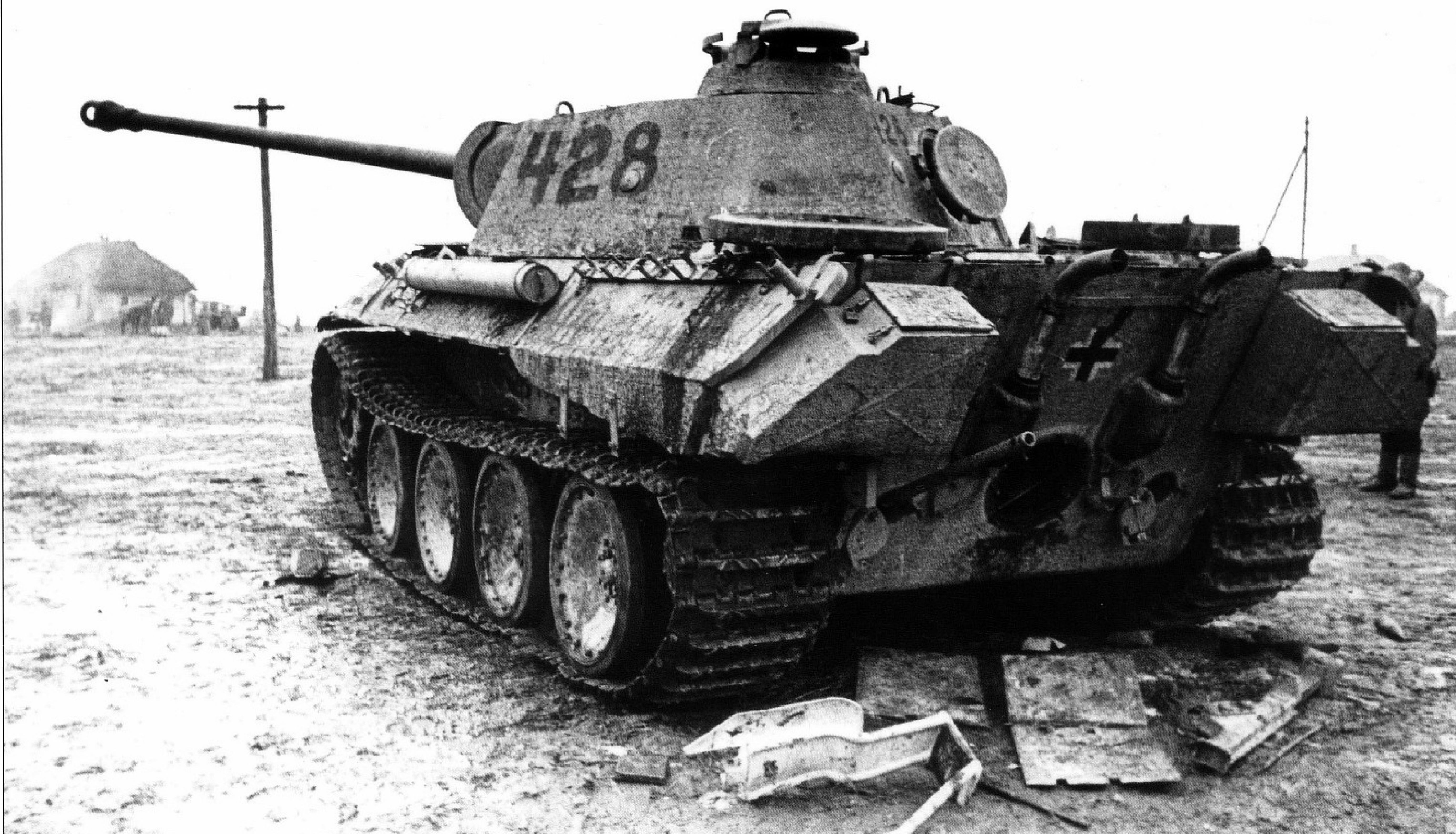
19- This winter 1943/44 captured Ausf. A does not show any major external damage. Note that this tank has an improved commander's cupola installed. As it was common with most Ausf. A, this tank's vertical surfaces have been covered in Zimmerit compound. The turret tactical numbers have been hastily painted on by the former owners. (S. Netrebenko)
