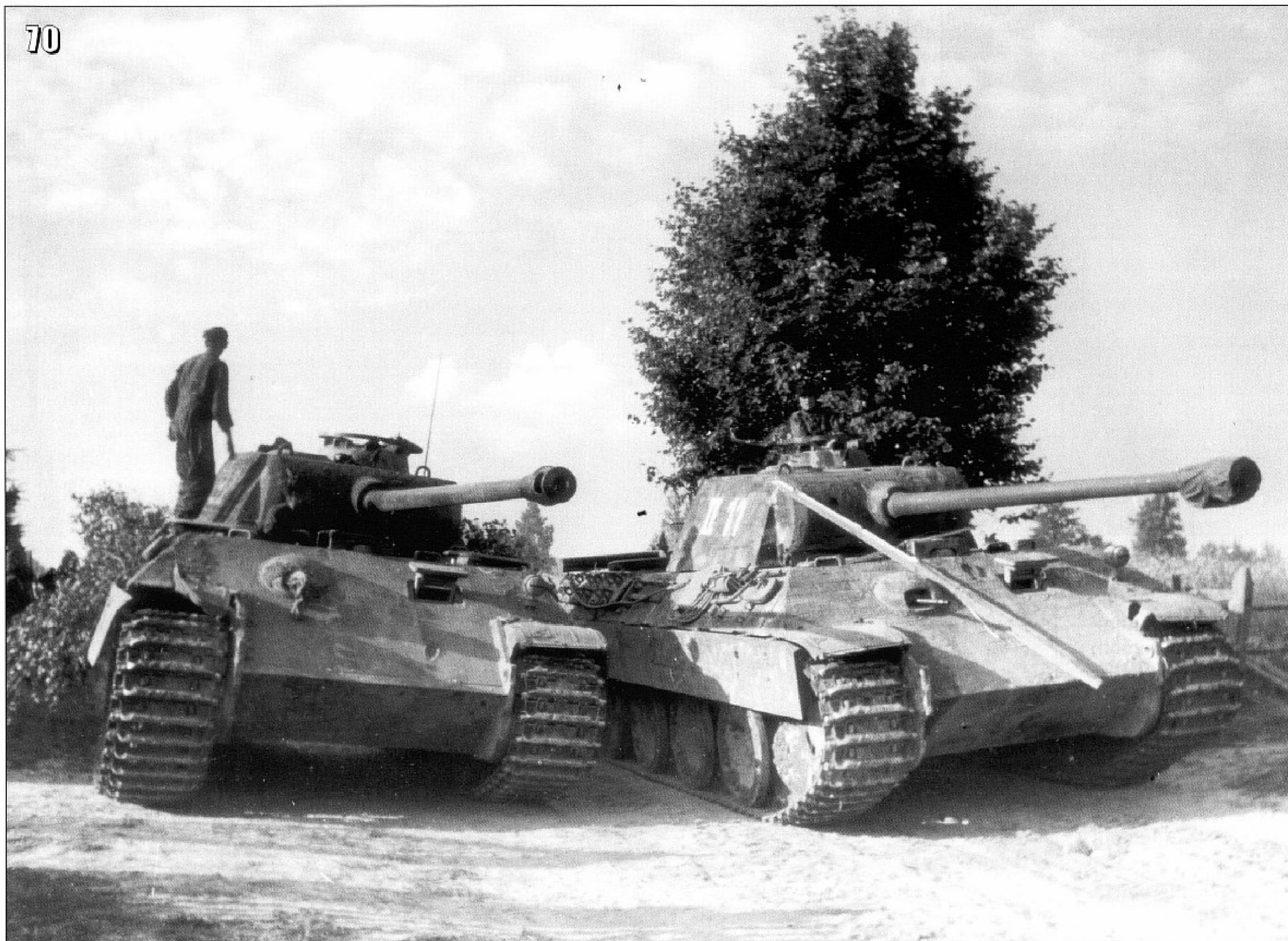
70- The Panther on the left was hit on the front glacis plate. The tilted tank indicates that there might be more damage to the left running gear. Trying to repair this tank on the spot looks impossible. Another Panther, also an Ausf. A, being driven up to attempt towing. (Anderson)
