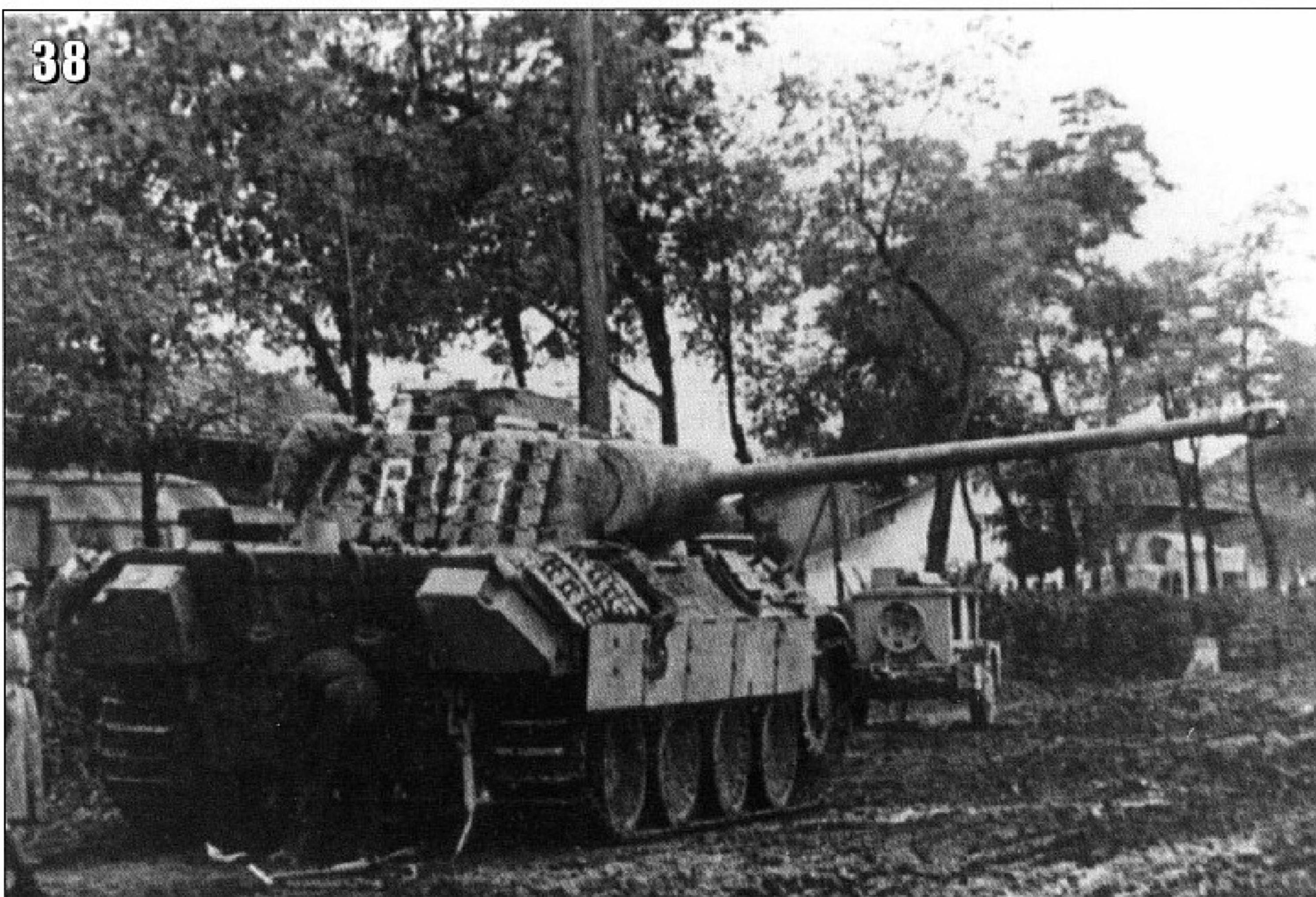
38- The Commander's "mount" is undergoing some repair. The tactical code "R01" has been painted on the spare track sections carried on the turret sides. The empty radiant directing aerial mast base is visible on the engine deck. This photo was shot in Hungary in late Summer 1944. (Anderson)
